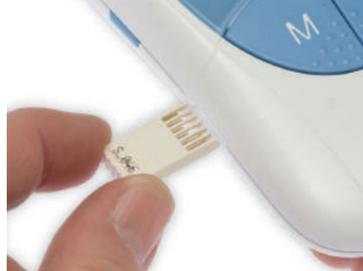
Make sure the meter is off. With the code number facing up, insert the code chip into the code chip slot until it snaps into place.
