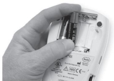
Insert 4 AAA batteries according to the diagram inside the battery compartment.
