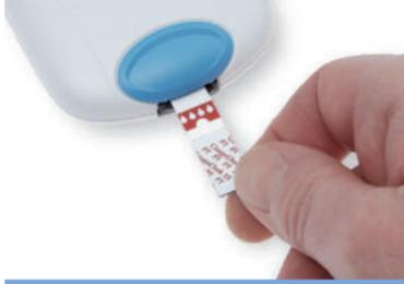
Slide the test strip into the test strip guide in the direction of the arrows until it stops.
